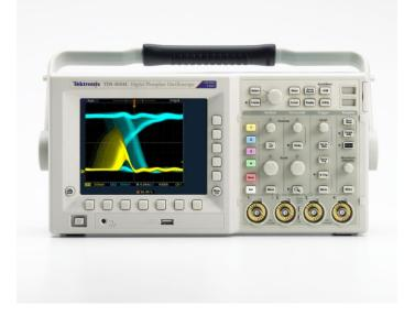
The TDS3000C Series provides you with the performance you need at a price you can afford. Bandwidths range from 100 MHz to 500 MHz, with up to 5 GS/s sample rates for accurate representation of your signal.
